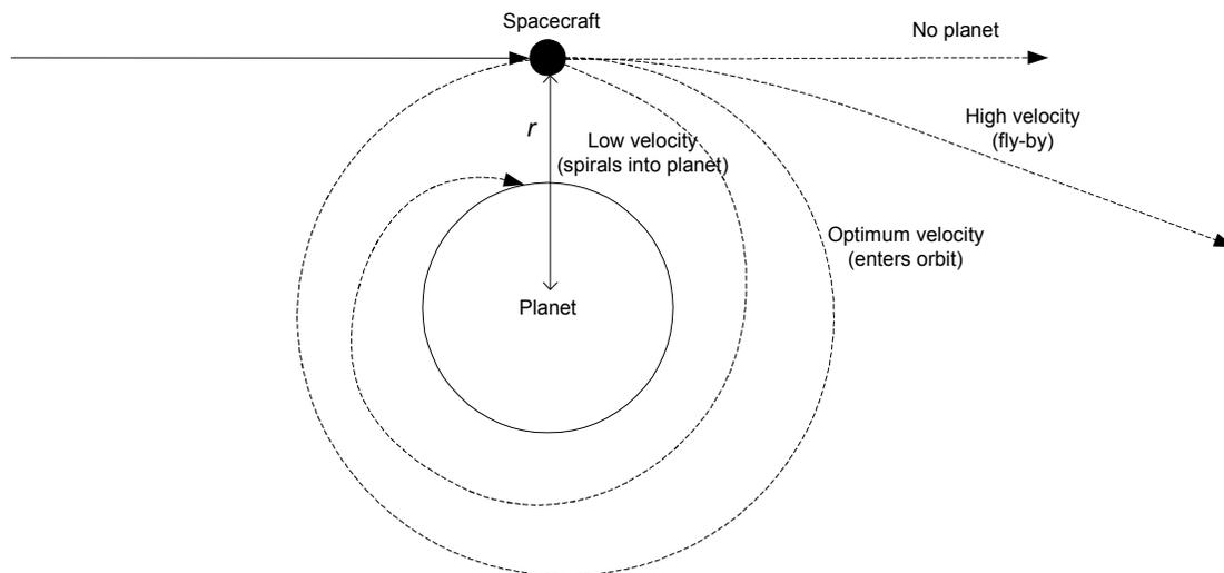
One way of thinking about this is that the curvature of the planet is such that it falls away at the same rate as gravity is pulling the spacecraft towards it. The spacecraft is in “free fall” around the planet.
