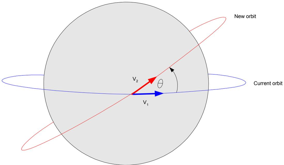
As the satellite is staying at the same altitude we know that the magnitude of the velocity vectors  $v_1$  and  $v_2$  will be the same, but the direction will be different. To work out the velocity vector  $\Delta V$  to effect a change the direction through an angle  $\theta$  we simply construct a vector triangle.
