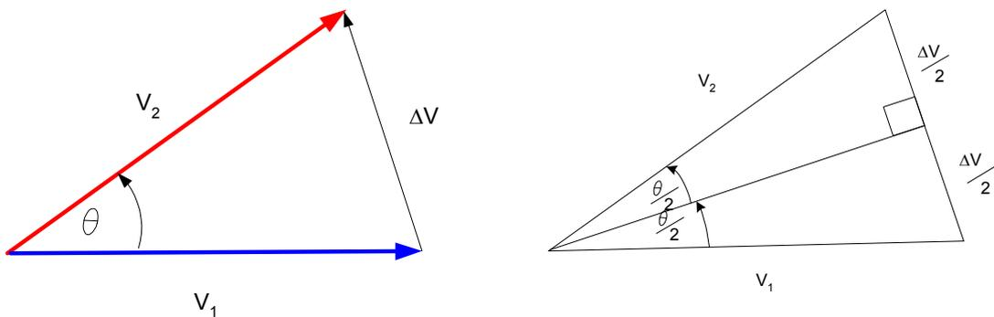
Applying simple trigonometry to the velocity we can show that the magnitude of the velocity vector  $\Delta V$  is:
