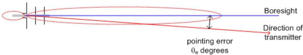
For small pointing errors, defined as angles which are less than half the -3dB beamwidth, the pointing loss can be approximated to:
